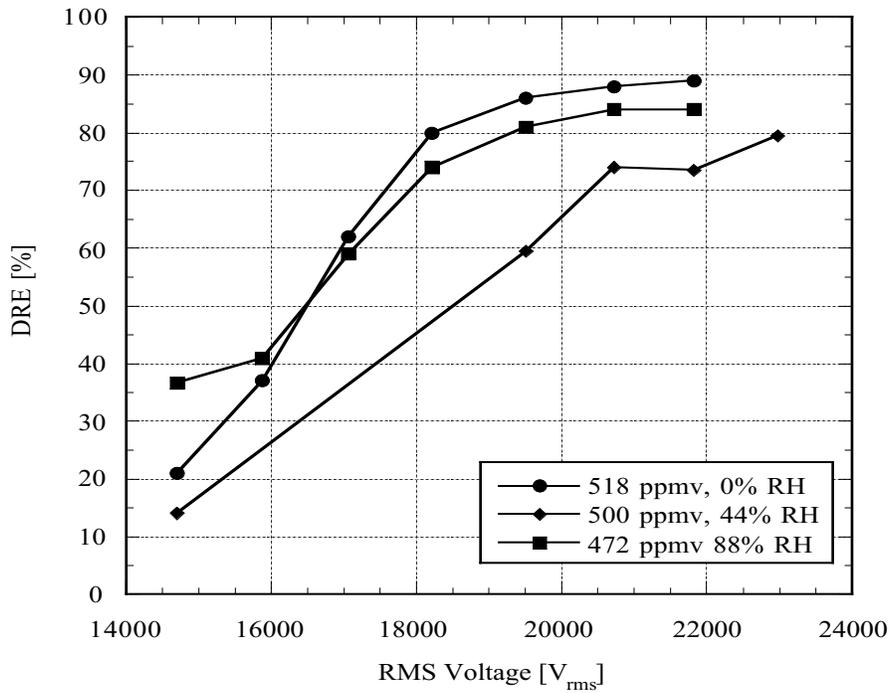
**Figure 4. Effect of Relative Humidity on the DRE of 500 ppmv Benzene in Air in Cylindrical Dielectric Barrier Discharge Plasma Reactor. Gas residence time = 0.68 min, T = 293 K, P = 0.85 atm.**
