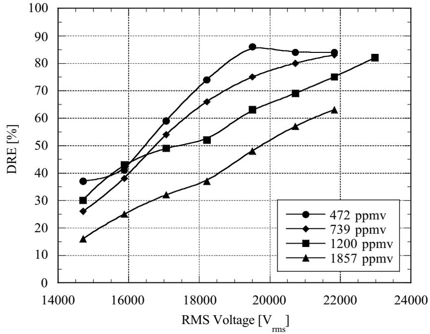
**Figure 3. Destruction Removal Efficiencies for Benzene in Air in Cylindrical Dielectric Barrier Discharge Plasma Reactor at 88% Relative Humidity. Gas residence time = 0.68 min, T = 293 K, P = 0.85 atm.**
