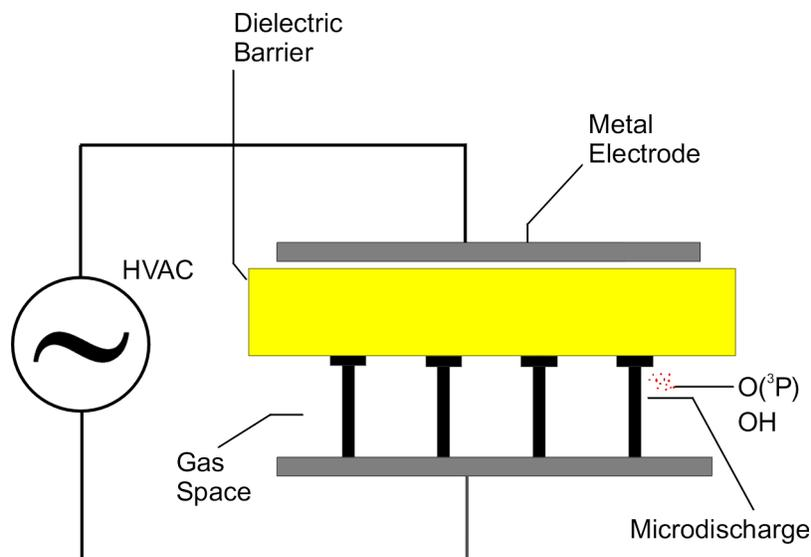
**Figure 1. Planar, Single Dielectric Barrier Discharge Reactor.**
