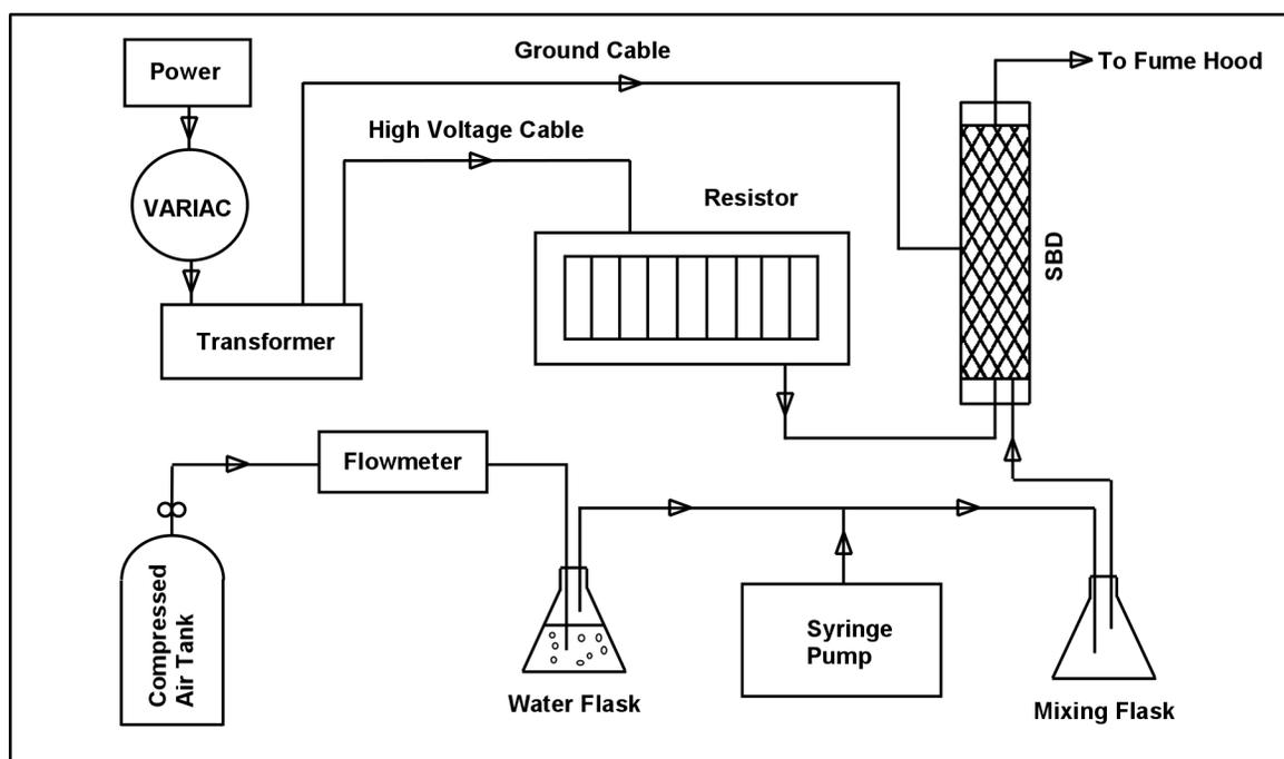
**Figure 2. Schematic for Cylindrical Dielectric Barrier Discharge Plasma Reactor System.**
